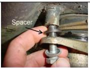
7 – Install spring plates with torsion bars.
